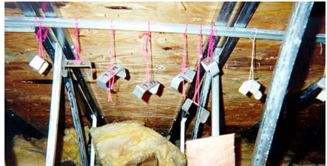
Figure 3 - Attic Specimens in Miami, Florida Site
